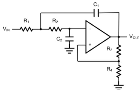
**Figure 9. Sallen-Key 2nd Order Active Low-Pass Filter**
