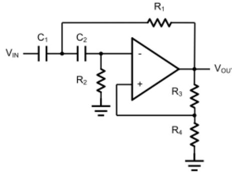
**Figure 10. Sallen-Key 2nd Order Active High-Pass Filter**
