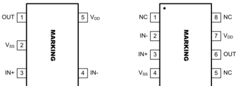
**Figure 1. Pin Assignment Diagram (SOT23-5 and SOP8 Package)**
