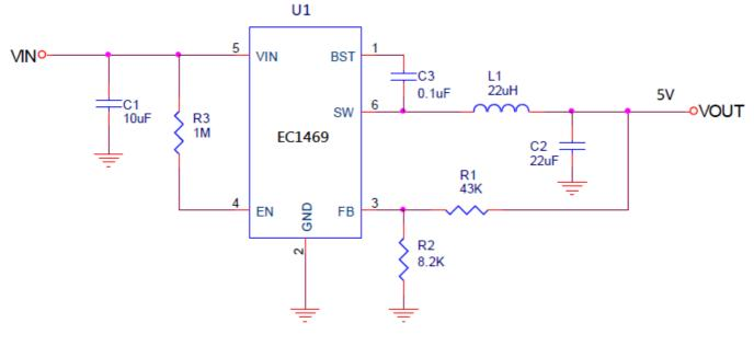
$V_{OUT} = V_{REF}(1 + \frac{R1}{R2})$
