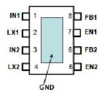
Figure 2 Pin Configuration of EC3221
