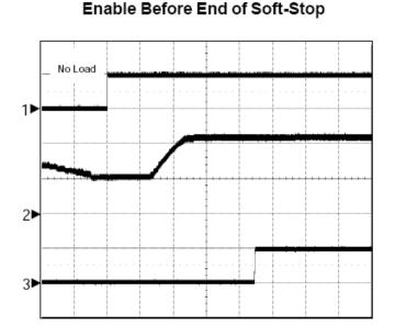
CH1: V<sub>EN</sub>, 5V/Div, DC CH2: V<sub>OUT</sub>, 500mV/Div, DC CH3: V<sub>POK</sub>, 5V/Div, DC TIME: 500μs/Div
