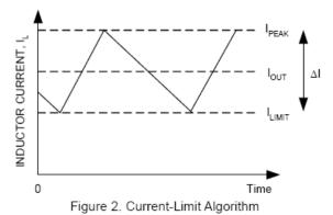
The PWM controller uses the low-side MOSFETs on-resistance RDS(ON) to monitor the current for protection against shortened outputs. The MOSFET's RDS(ON) is varied by temperature and gate to source voltage, the user should determine the maximum RDS(ON) in manufacture's datasheet.
