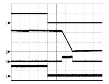
CH1: V<sub>EN</sub>, 5V/Div, DC CH2: V<sub>OUT</sub>, 500mV/Div, DC CH3: V<sub>LGATE</sub>, 5V/Div, DC CH4: V<sub>POK</sub>, 5V/Div, DC TIME: 5ms/Div
