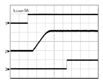
CH1: V<sub>EN</sub>, 5V/Div, DC CH2: V<sub>OUT</sub>, 500mV/Div, DC CH3: V<sub>POK</sub>, 5V/Div, DC TIME: 500µs/Div
