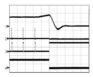
CH1: V<sub>OUT</sub>, 1V/Div, DC CH2: V<sub>UGATE</sub>, 20V/Div, DC CH3: V<sub>LGATE</sub>, 5V/Div, DC CH4: V<sub>POK</sub>, 5V/Div, DC TIME: 50µs/Div
