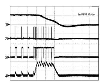
CH1: V<sub>OUT</sub>, 1V/Div, DC CH2: V<sub>UGATE</sub>, 20V/Div, DC CH3: V<sub>LGATE</sub>, 5V/Div, DC CH4: I<sub>L</sub>, 20A/Div, DC TIME: 20µs/Div
