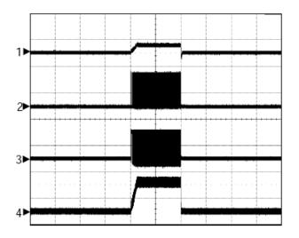
CH1: V<sub>OUT</sub>, 1V/Div, DC CH2: V<sub>UGATE</sub>, 20V/Div, DC CH3: V<sub>LGATE</sub>, 5V/Div, DC CH4: I<sub>L</sub>, 20A/Div, DC TIME: 1ms/Div
