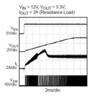
Figure 7. Startup Through Enable
