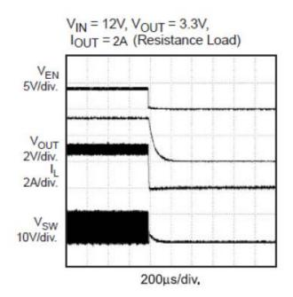
Figure 9. Shutdown through Enable
