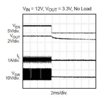
Figure 8.Shutdown through Enable
