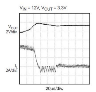
Figure 12. Short Circuit Recovery
