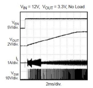
Figure 6. Start up through Enable
