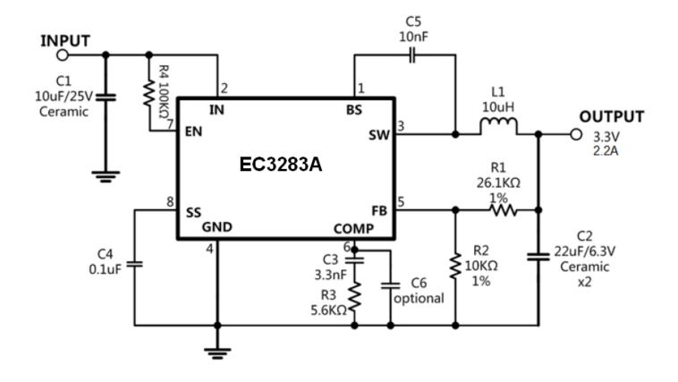
Fig13. EC3283A with 3.3V Output, 22µF/6.3V Ceramic Output Capacitor
