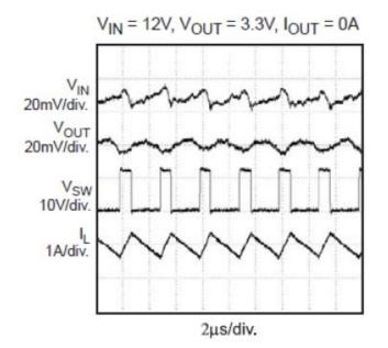
Figure 4. Steady State Test
