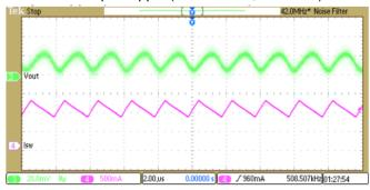
Output Ripple (12V => 3.3V, Load=2A)
