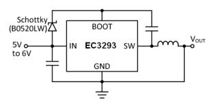
Figure 2: Add a Schottky diode to promote efficiency when  $V_{IN} \le 6V$ .
