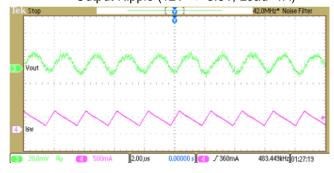
Output Ripple (12V => 3.3V, Load=0A)
