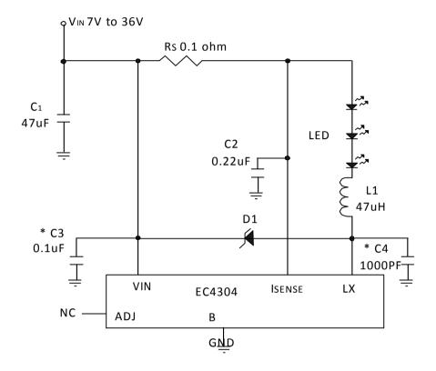
\* note: When outputs the big current, the noise are big, this and the system environment and PCB layout have the influential, may defer to the actual need to increase the capacitor filtration noise.
