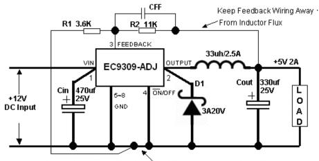
Heavy Lines Must Be Kept Short And Use Ground Plane Construction For Best Results
