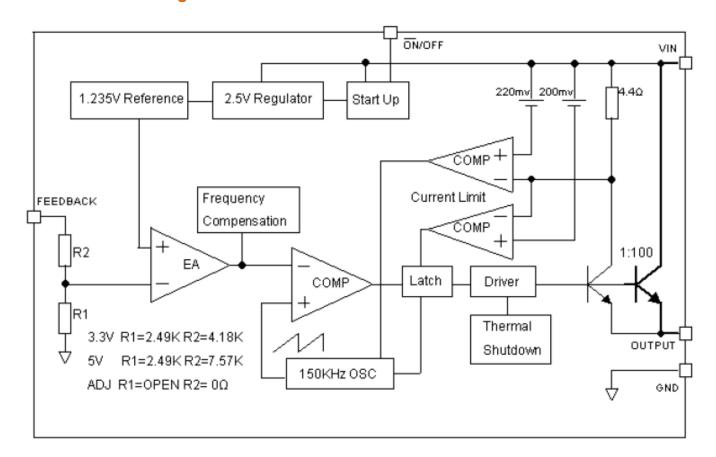
Figure 3 Function Block Diagram of EC9309
