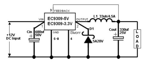
Figure 11. Typical Application of EC9309 For 3.3V & 5V
