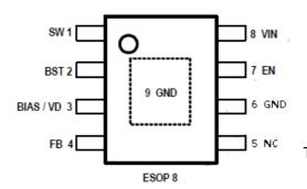
The pad and Pin-6 must be connected to GND.
