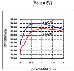
Efficiency vs Load Current
