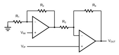
Figure 6. Two-Op-Amp Instrumentation Amplifier
