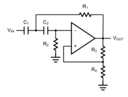
Figure 10. Sanllen-Key 2nd Order Active High-Pass Filter
