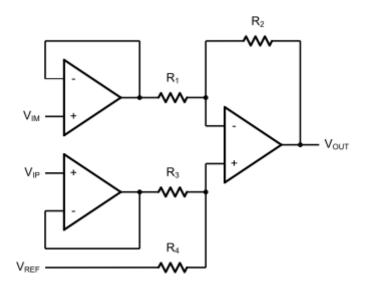
Figure 5. Three-Op-Amp Instrumentation Amplifier
