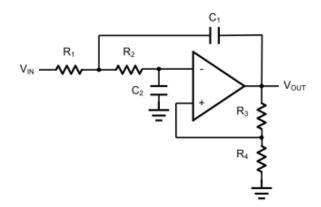
Figure 9. Sanllen-Key 2nd Order Active Low-Pass Filter
