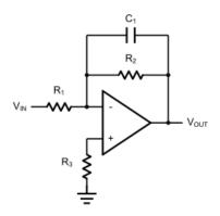
Figure 8. Low Pass Active Filter
