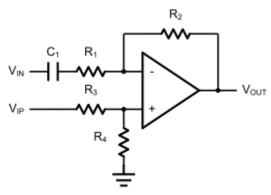
Figure 7. Single Supply Inverting Amplifier
