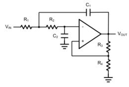
Figure 9. Sanllen-Key 2nd Order Active Low-Pass Filter
