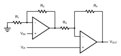
Figure 6. Two-Op-Amp Instrumentation Amplifier
