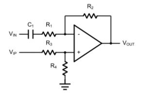
Figure 7. Single Supply Inverting Amplifier
