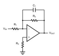
Figure 8. Low Pass Active Filter
