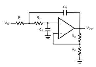
Figure 9. Sanllen-Key 2nd Order Active Low-Pass Filter
