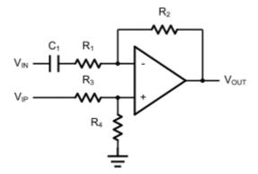
Figure 7. Single Supply Inverting Amplifier
