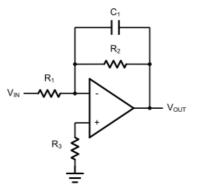
Figure 8. Low Pass Active Filter
