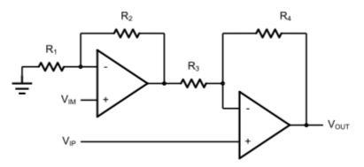
Figure 6. Two-Op-Amp Instrumentation Amplifier
