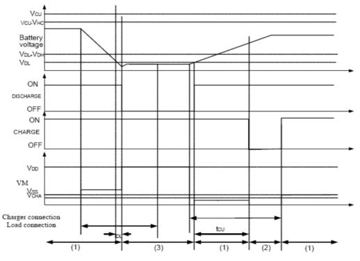
Remark: (1) Normal condition (2) Over-charge Voltage condition (3) Over-discharge Voltage condition (4) Over Current condition
