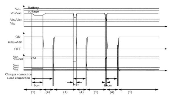
Remark: (1) Normal condition (2) Over-charge Voltage condition (3) Over-discharge Voltage condition (4) Over Current condition
