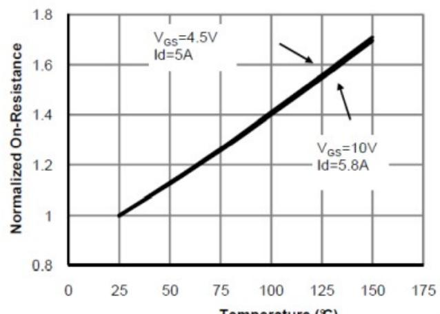
Figure 4: On-Resistance vs. Junction Temperature (Note E)
